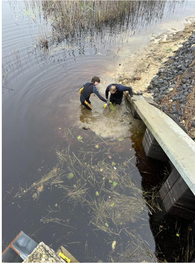
Photo 9: Divers wading and pouring concentrated dye at upstream end of lake side dam structure, end of northwest retaining wall. Multiple dye locations tested.
